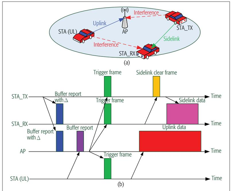
FIGURE 4. a) Sidelink and uplink transmissions can be performed concurrently if the received SINRs at both receivers are acceptable. b) The procedure of the proposed IEEE 802.11ax-based vehicular direct radio access.
