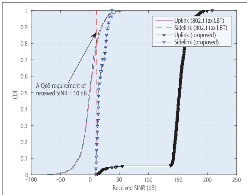
**FIGURE 5.** Simulation results of the proposed IEEE 802.11ax based vehicular direct radio access. In this simulation, the QoS requirements for the receiver of sidelink and the receiver of uplink both have SINR larger than 10 dB.
